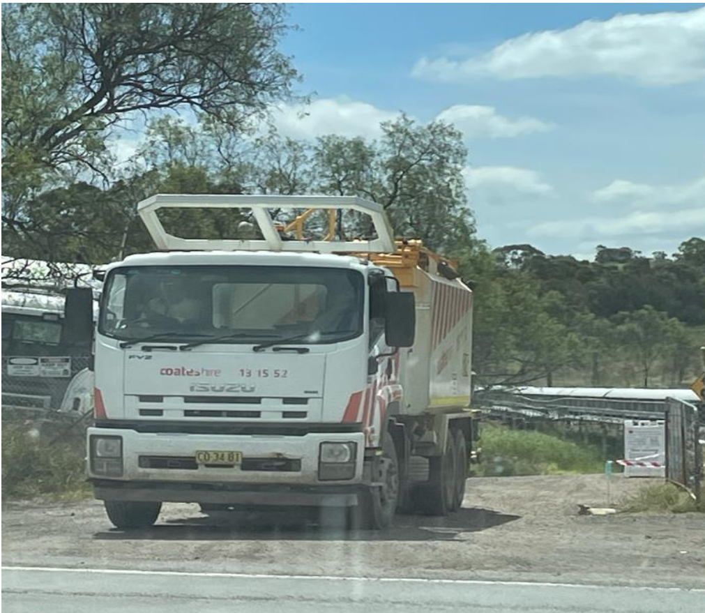
Plate 8 Water cart available on site for dust suppression
