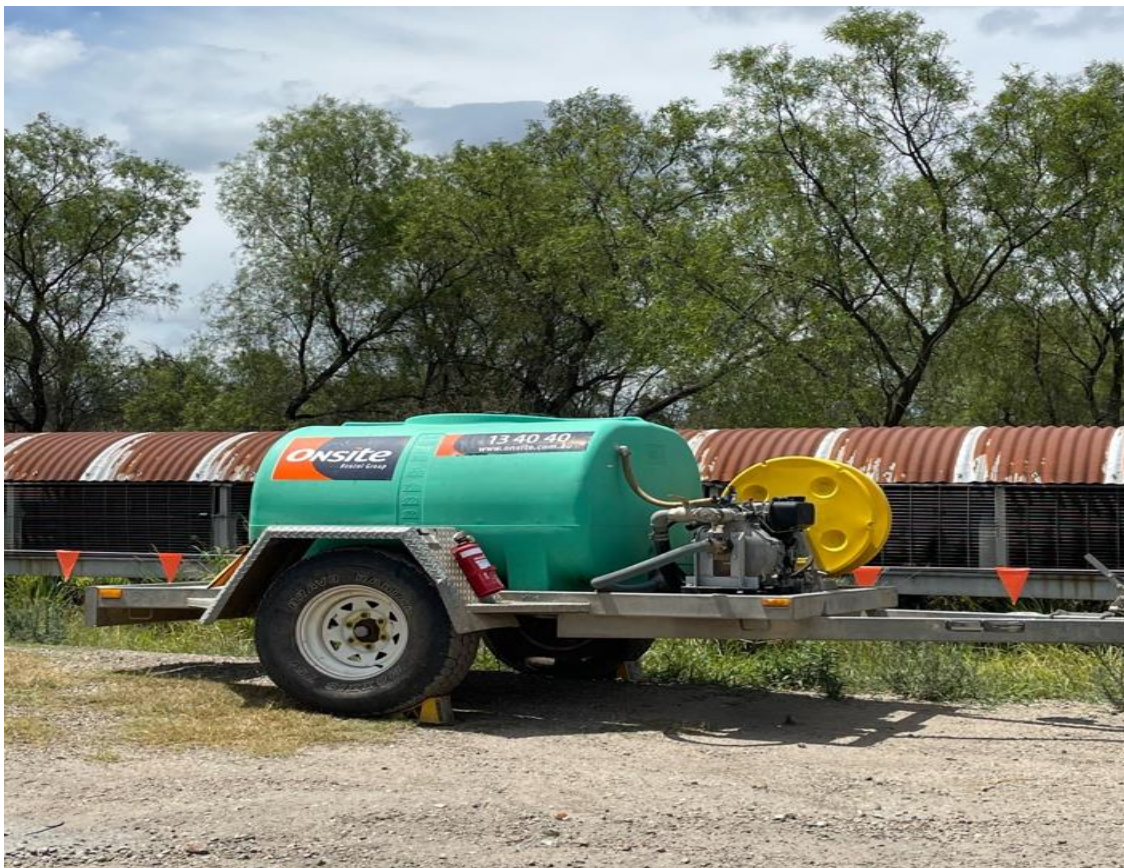
Plate 2 Fire suppression trailer
