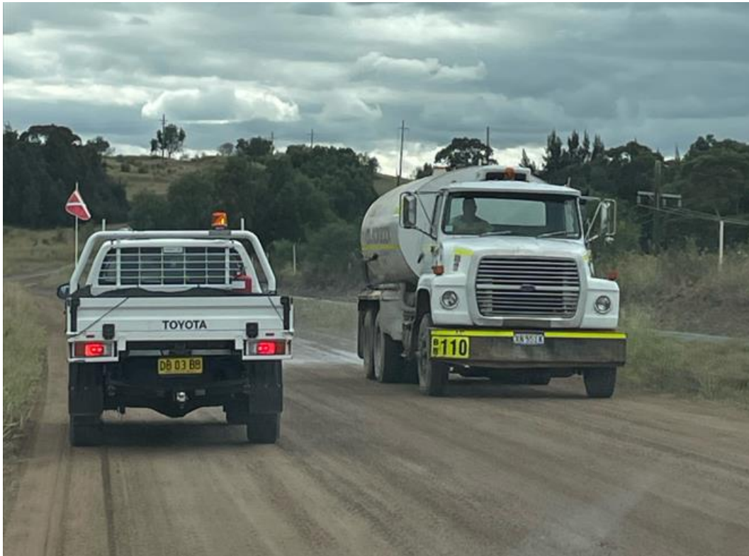
Plate 1 Water cart used on site for dust suppression
