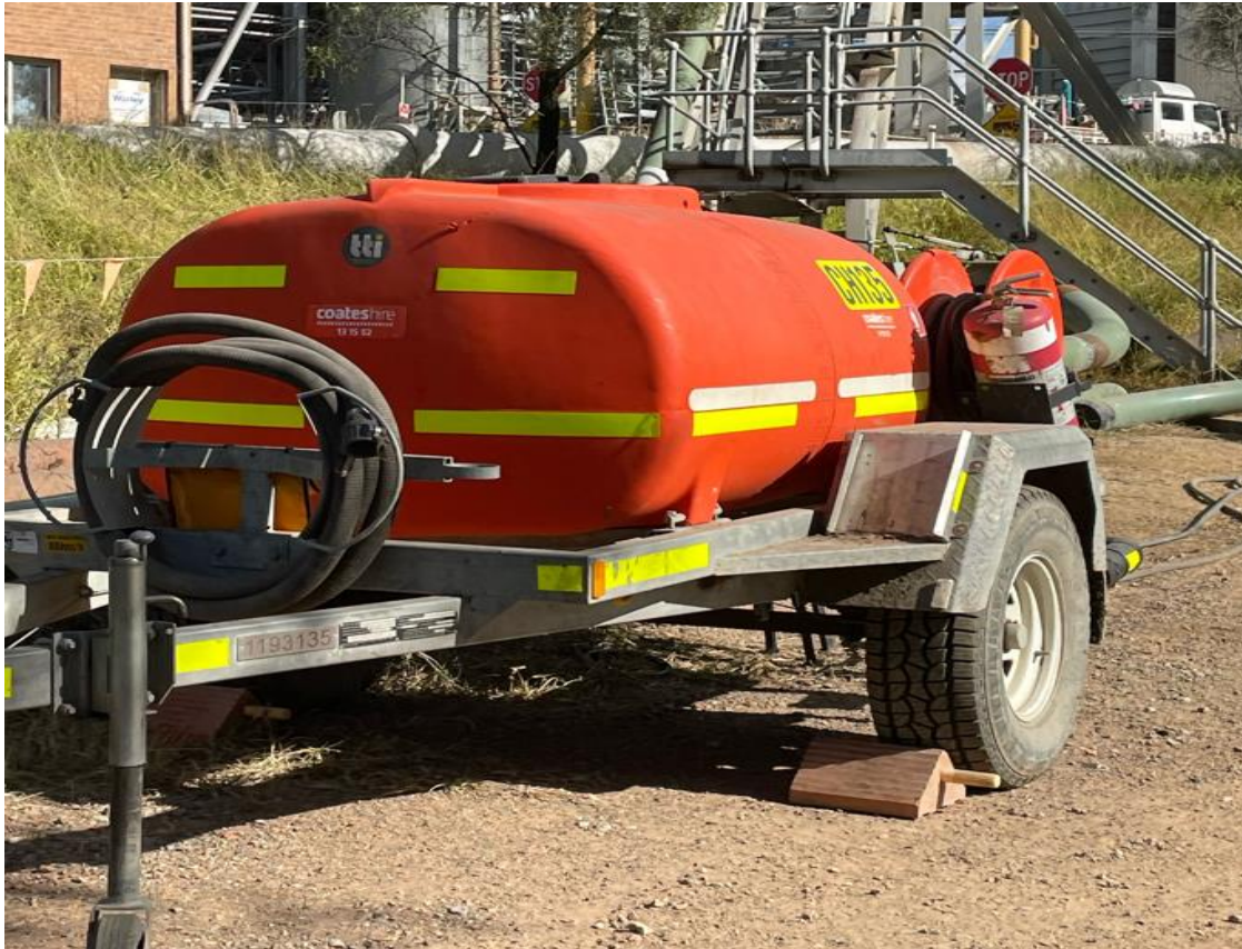
Plate 3 Fire suppression trailer
