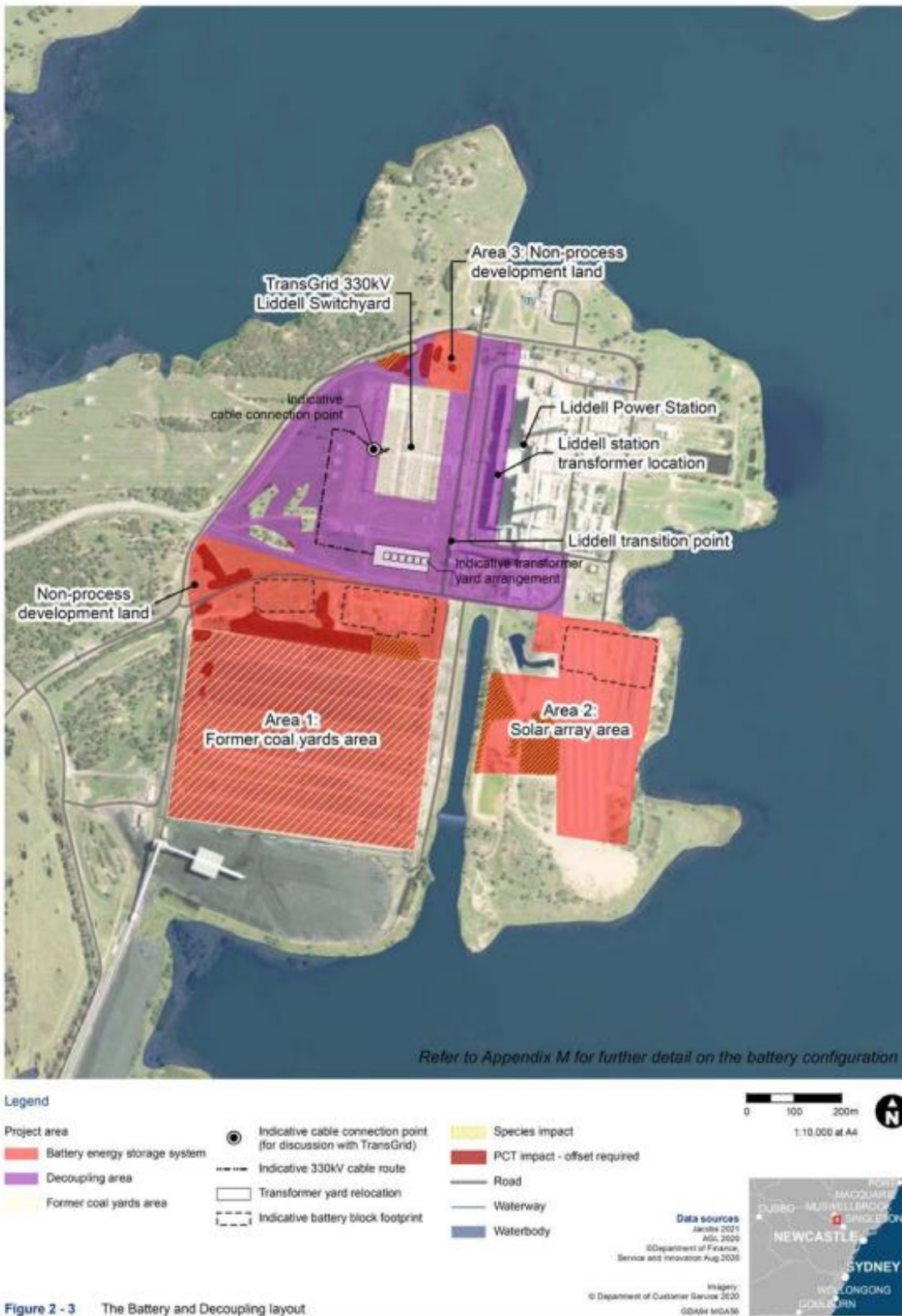
Figure 2 - 3 The Battery and Decoupling layout
