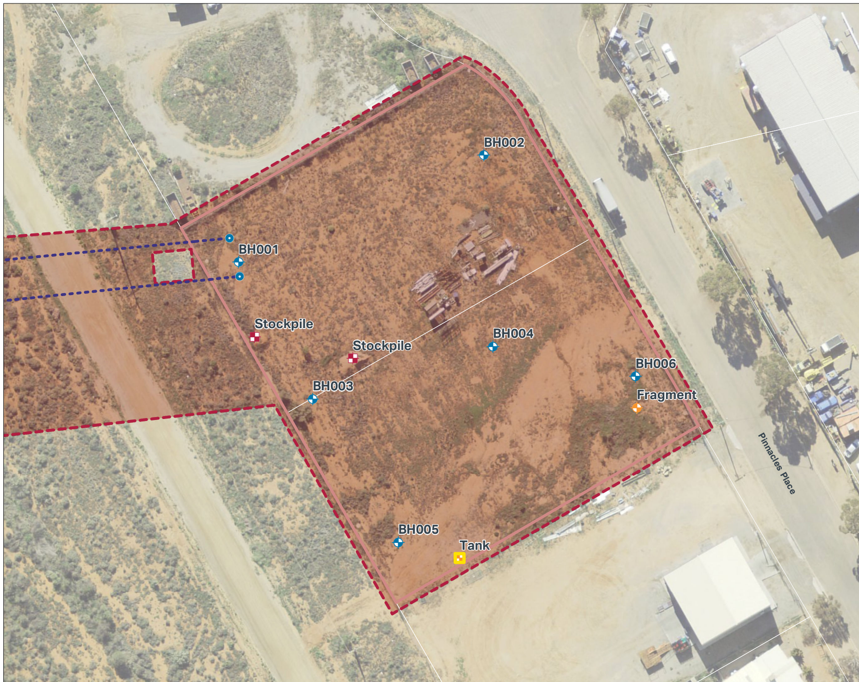
FIGURE A-3: BOREHOLE AND SAMPLING LOCATIONS
