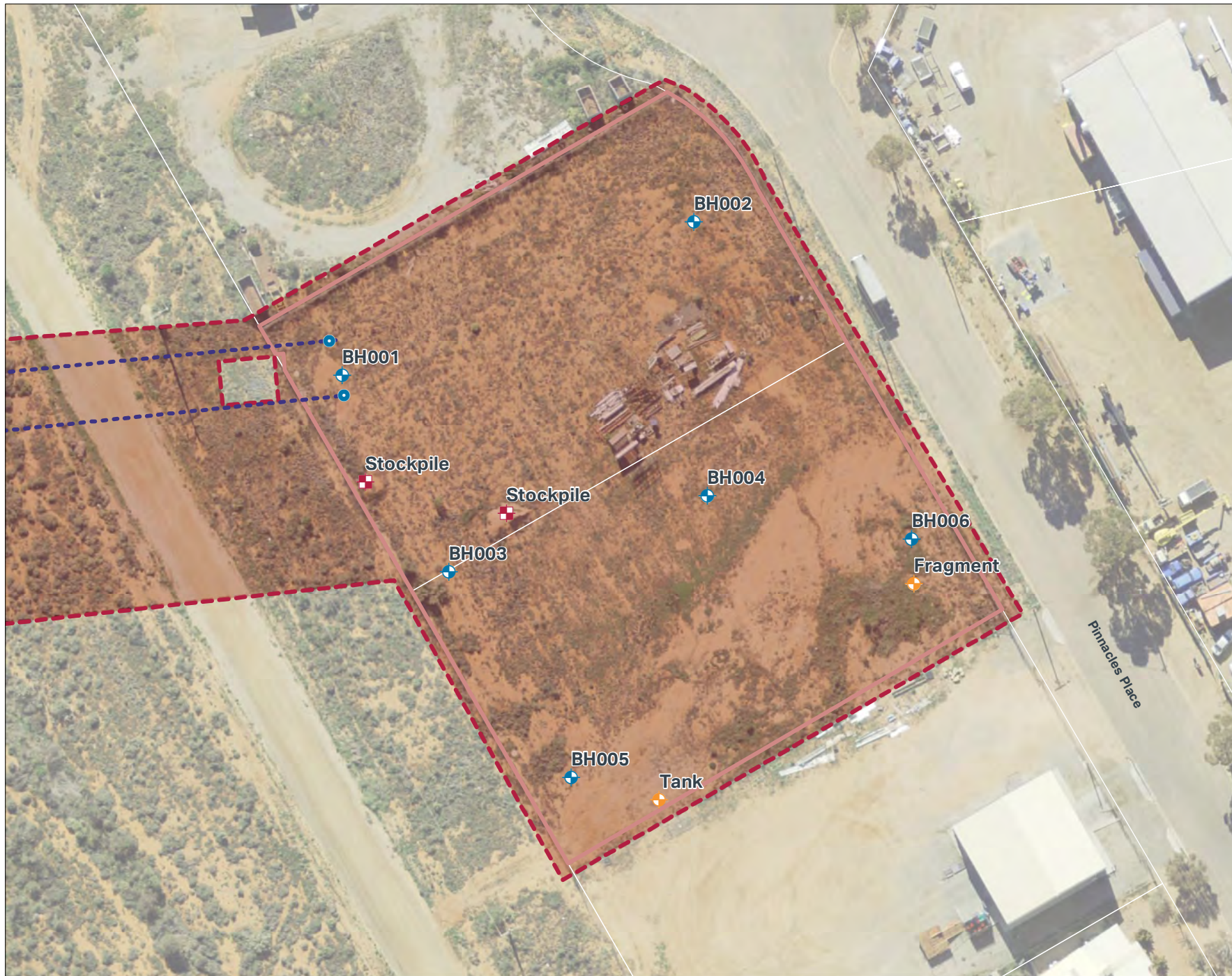
FIGURE 2: BOREHOLE AND SAMPLING LOCATIONS
