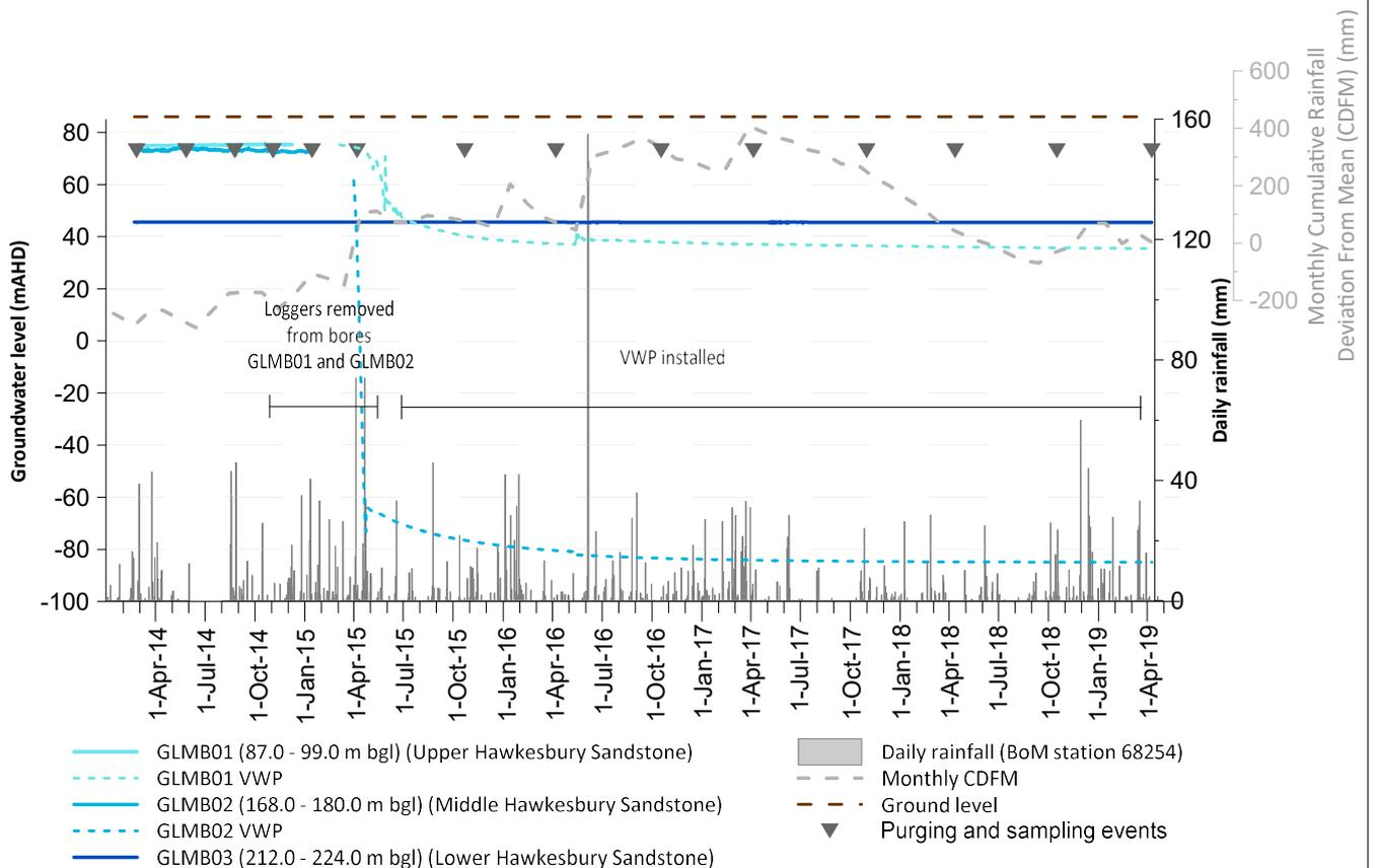
Although the absolute piezometric pressure values at GLMB01 and GLMB02 post-VWP installation are not representative of formation pressures, the trends in the data are and are therefore still useful.
