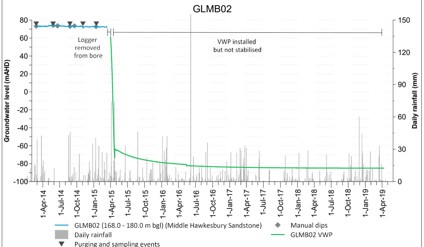
Although the absolute piezometric pressure values at GLMB01 and GLMB02 post-VWP installation are not representative of formation pressures, the trends in the data are and are therefore still useful.
