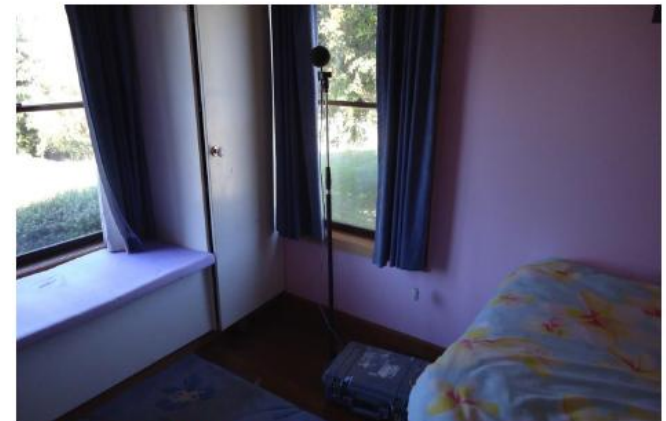
Figure A2 – Noise monitor installed in bedroom at Y21A
