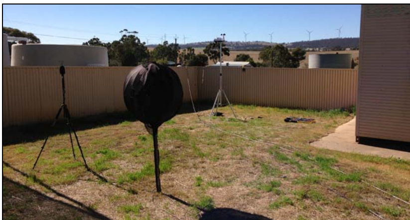
An infrasound (centre) and audio noise (left) monitoring site, with the meteorological station to the rear
