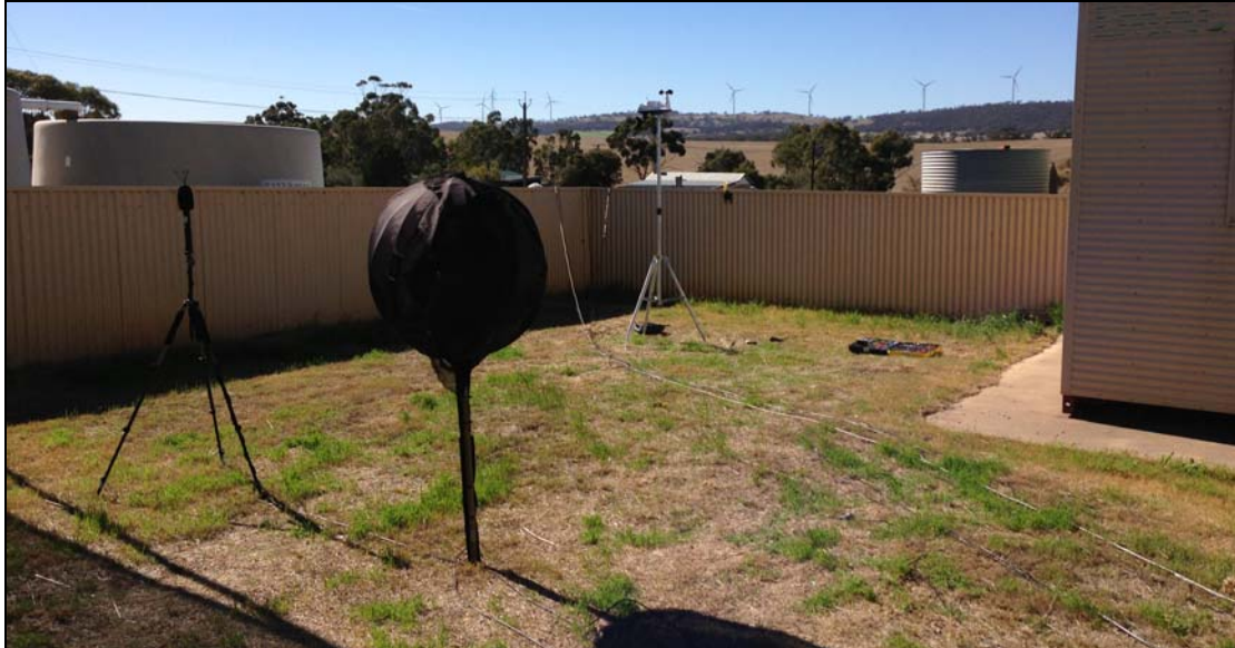
Figure 2 Monitoring station layout, showing an infrasound microphone with wind shield (centre), audio microphone (left) and the meteorological sensor
