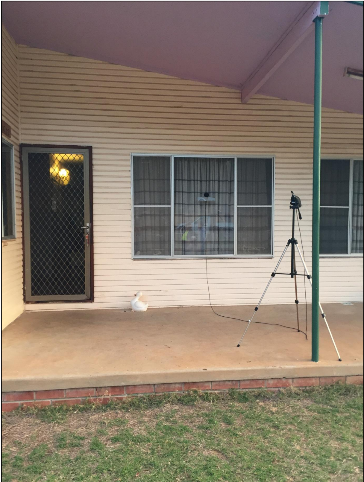
Figure 1 Example instrument microphone attached to the tested façade
