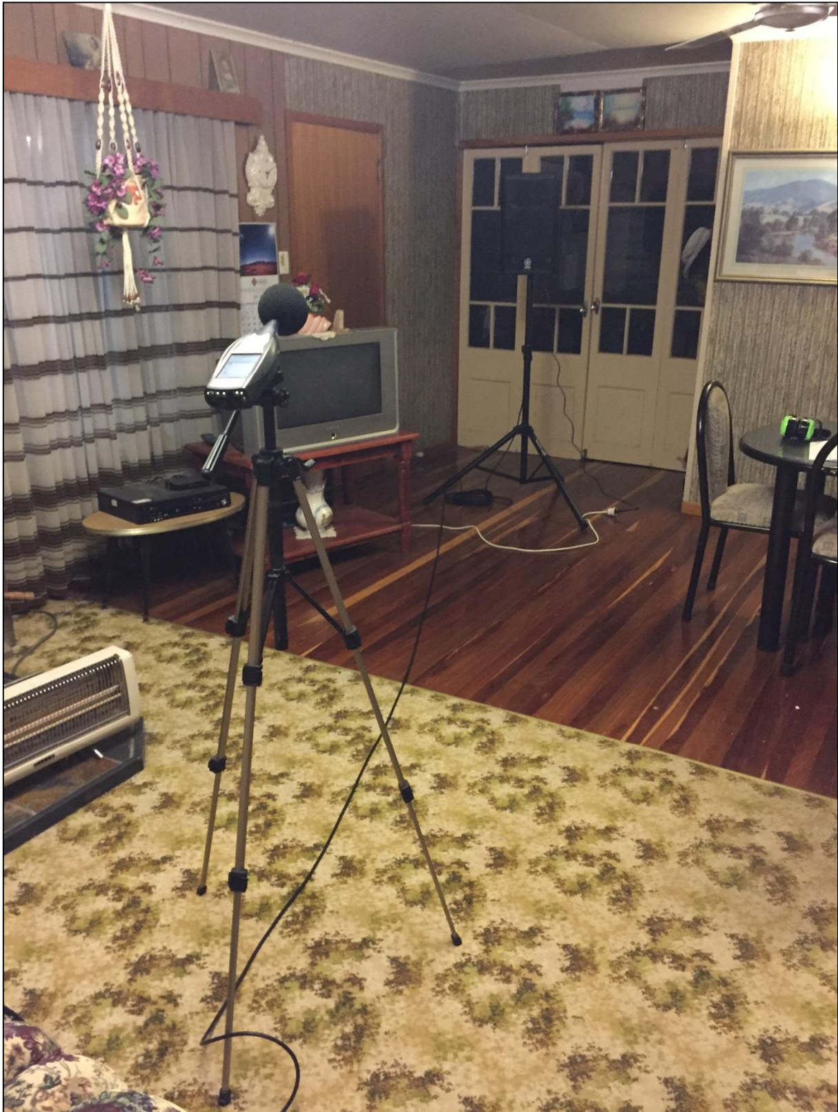
Figure 4 Example reverberation time measurement setup
