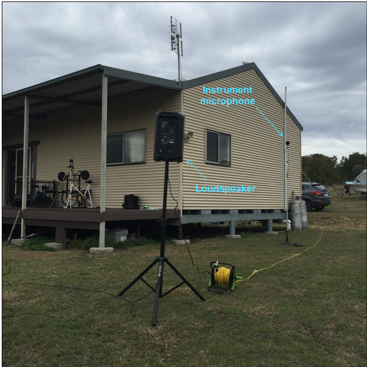
Figure 2 Example instrument microphone placed at 2m from façade and at 1.5m above finished floor level
