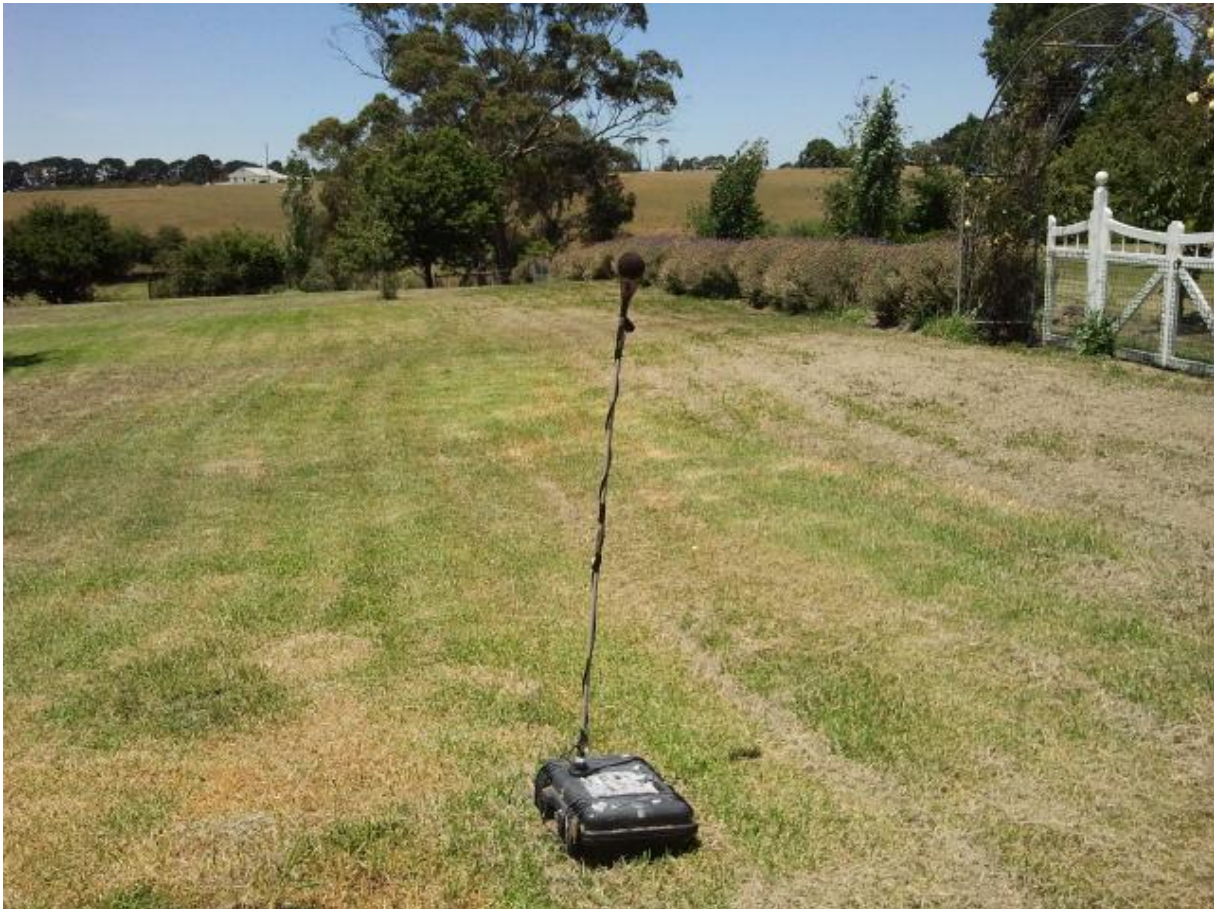
Figure 1 – Typical Noise Monitoring Installation
