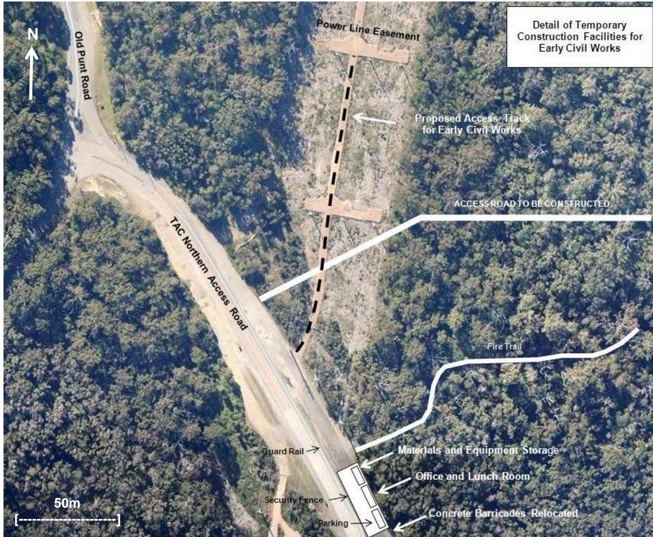
Figure 11-1: Site compound layout during early civil works
