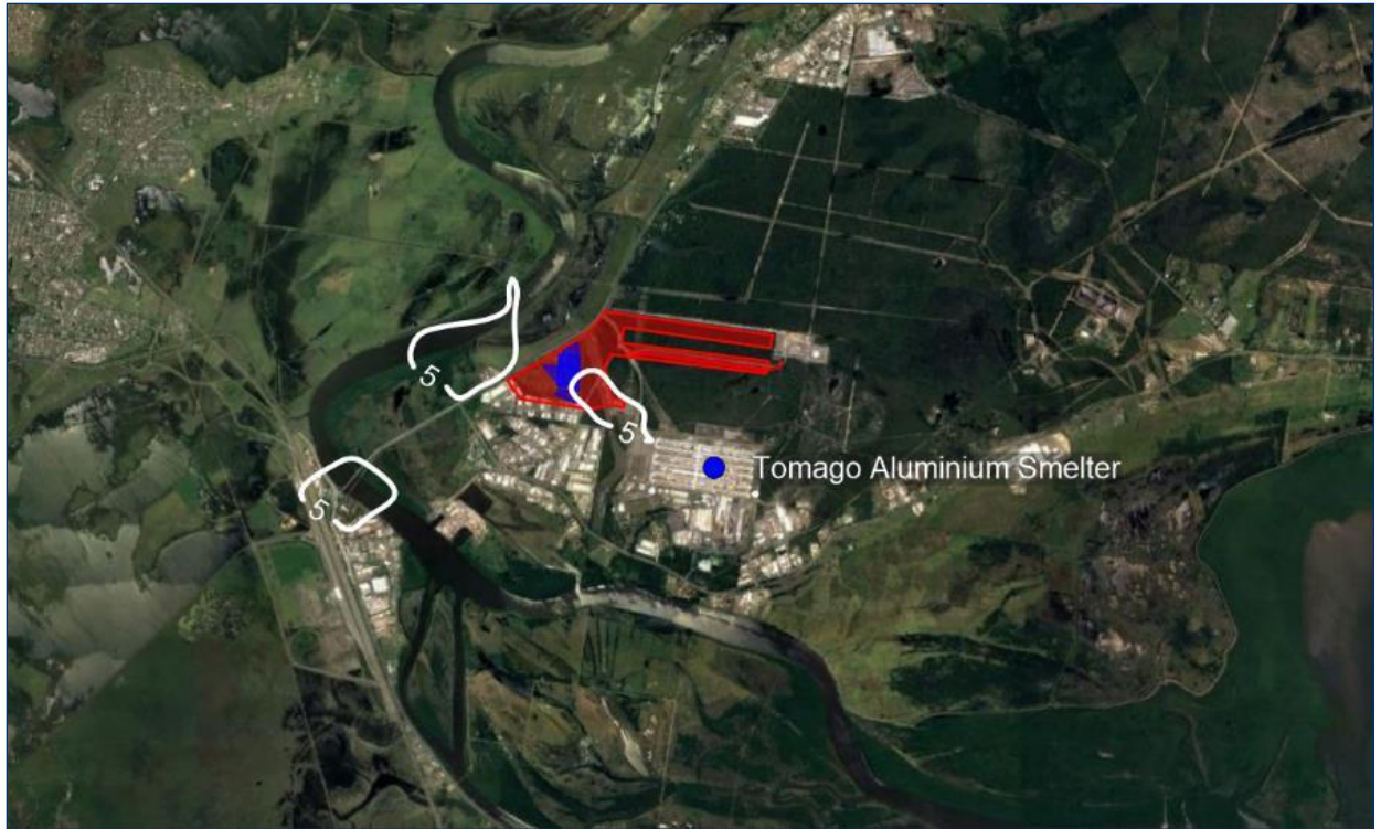
Figure 8.2: 99.9 th percentile 1 hour average SO 2 predictions, reciprocating engine, natural gas (µg/m 3 )
