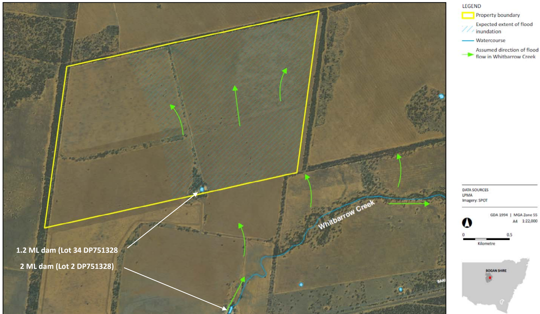
Figure 6-2 Inundation zones at the solar plant site.
