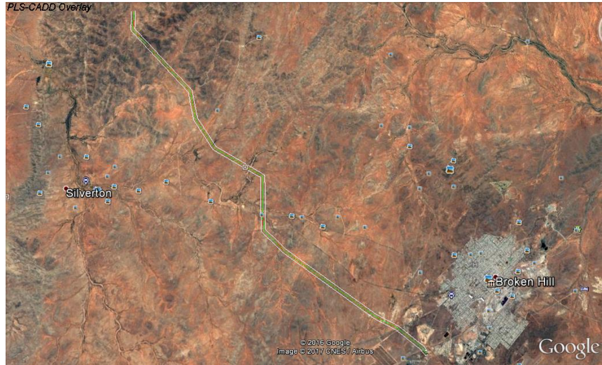
220kV Transmission Line route from TransGrid's existing Broken Hill 220kV substation to new Silverton Wind Farm 220kV Substation
