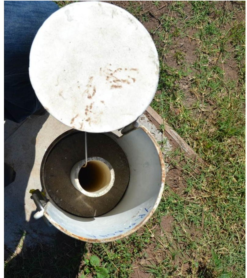
A water monitoring bore
