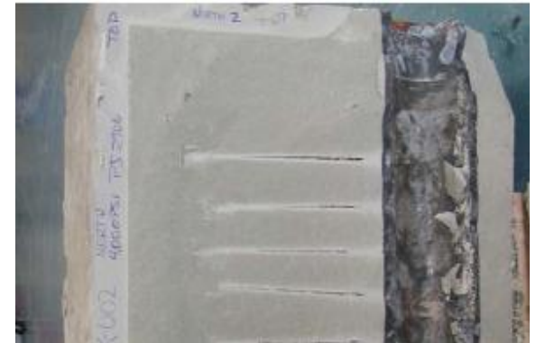
Cross section of perforated concrete
