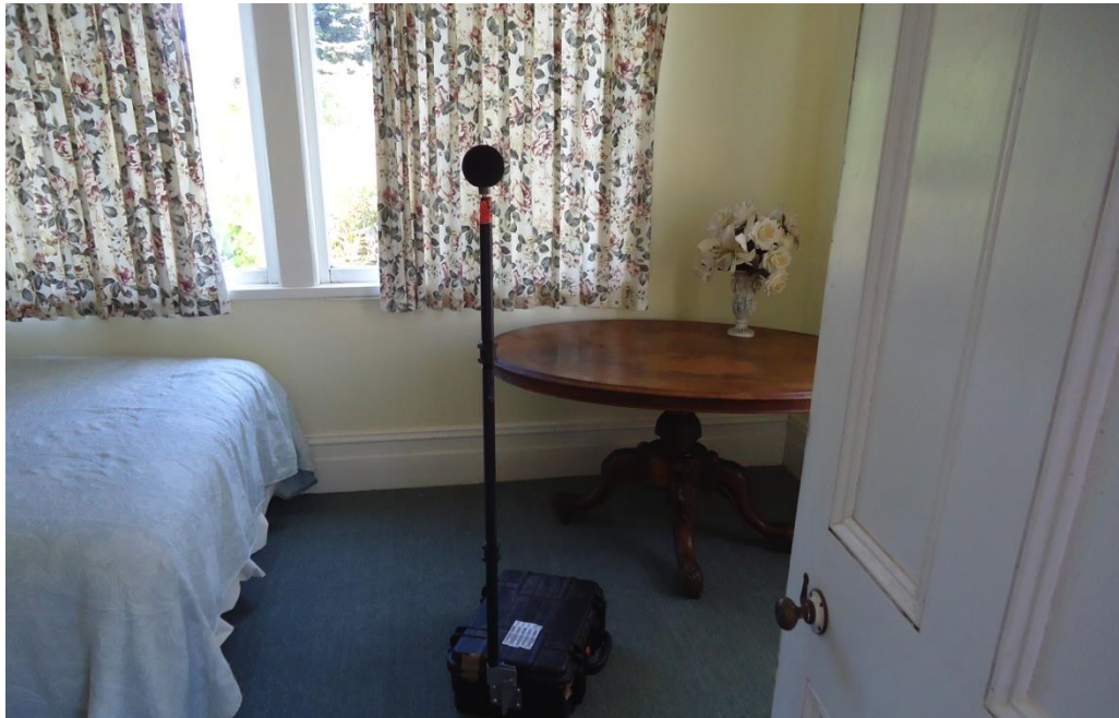
Figure A1 – Noise monitor installed in spare bedroom at O17A
