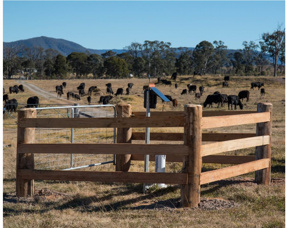
Water monitoring bore adjacent to Waukivory Pilot site
